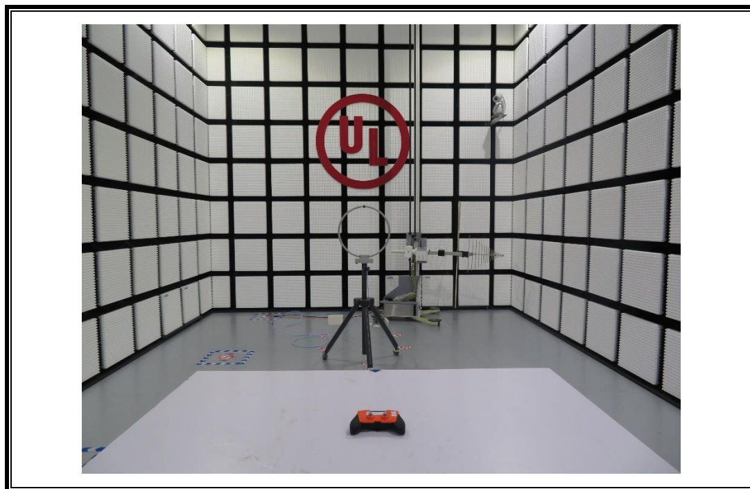
RADIATED RF MEASUREMENT SETUP (Below 30MHz)
