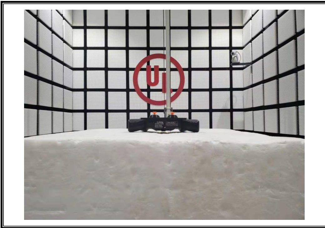
RADIATED RF MEASUREMENT SETUP (Above 1G – Y axis)
