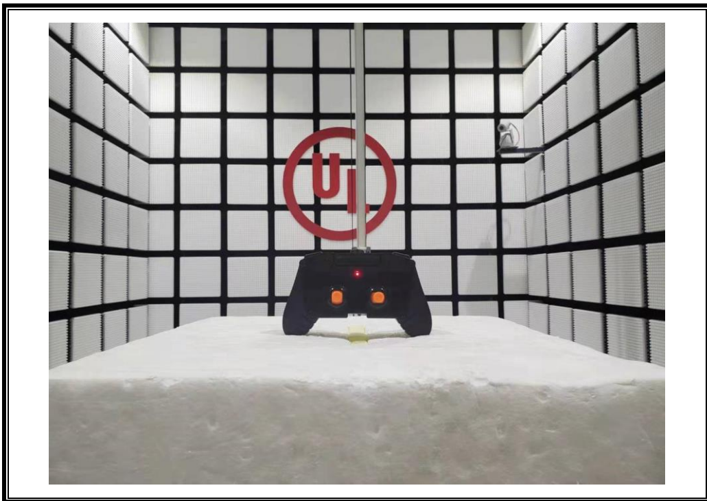
RADIATED RF MEASUREMENT SETUP (Above 1G – Y axis)
