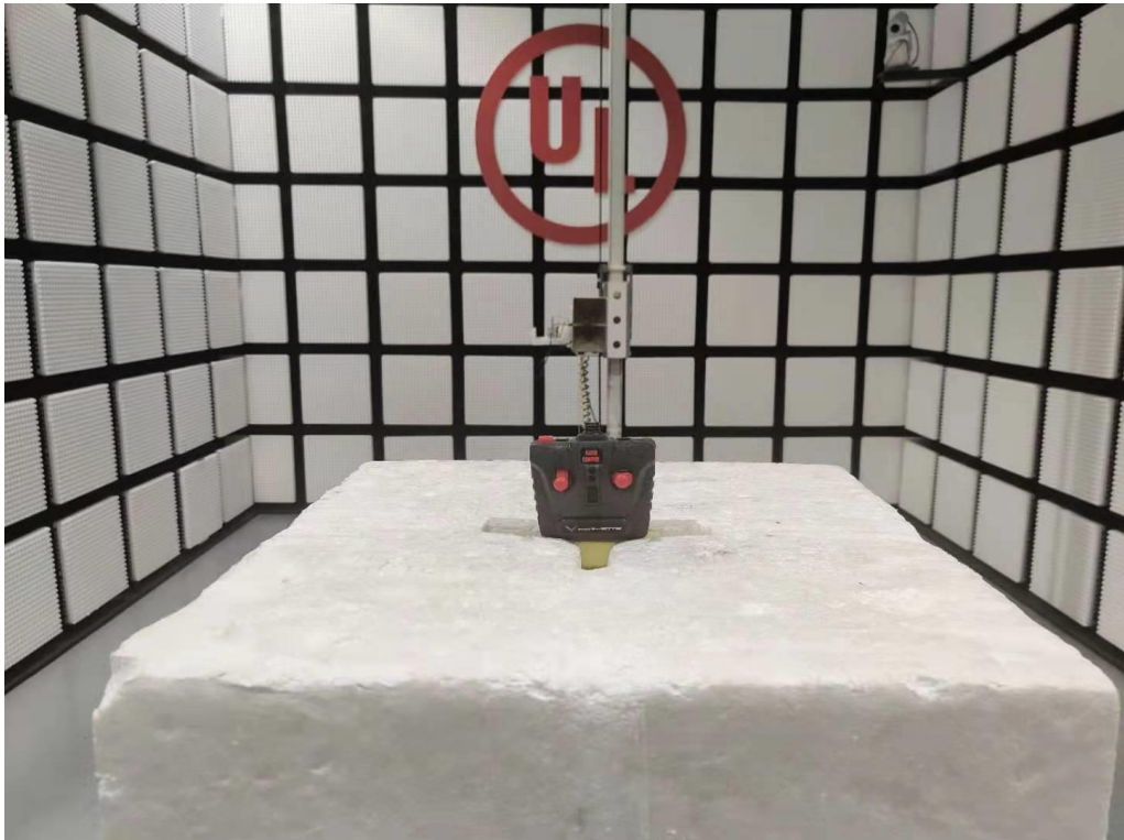
Radiated Disturbance Setup (Above 1 GHz – Y axis)
