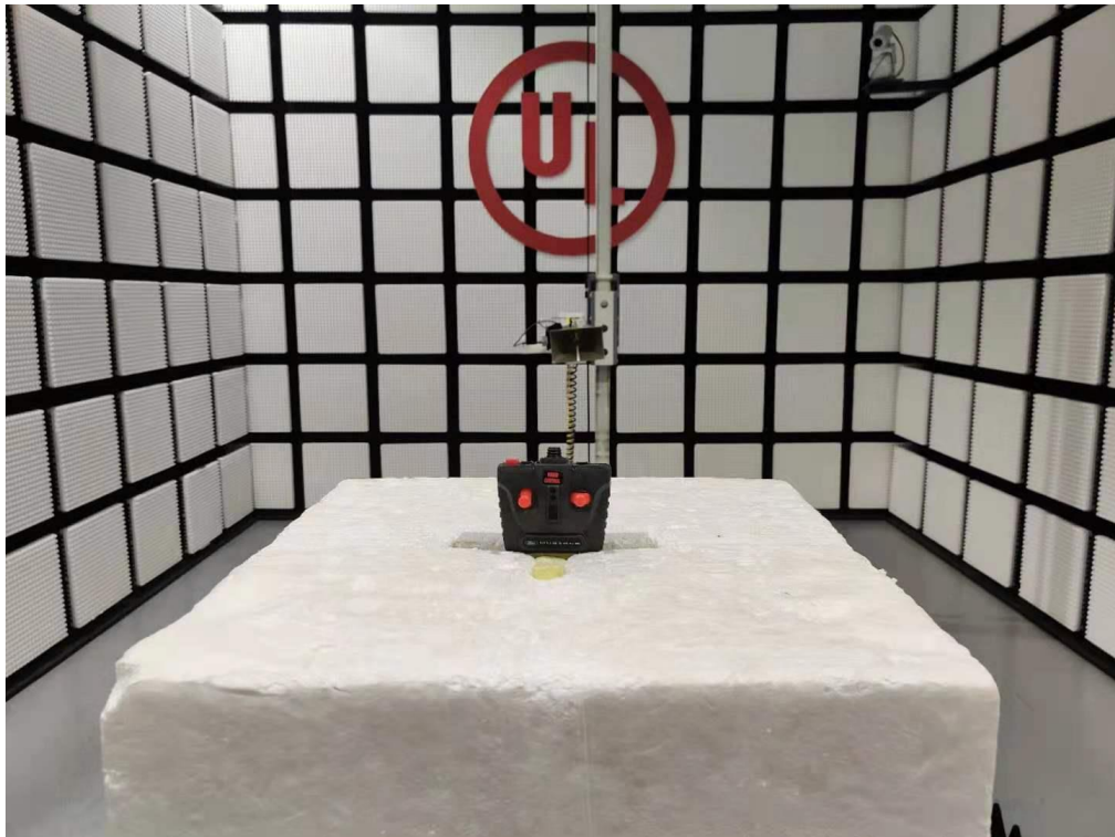
Radiated Disturbance Setup (Above 1 GHz – Y axis)
