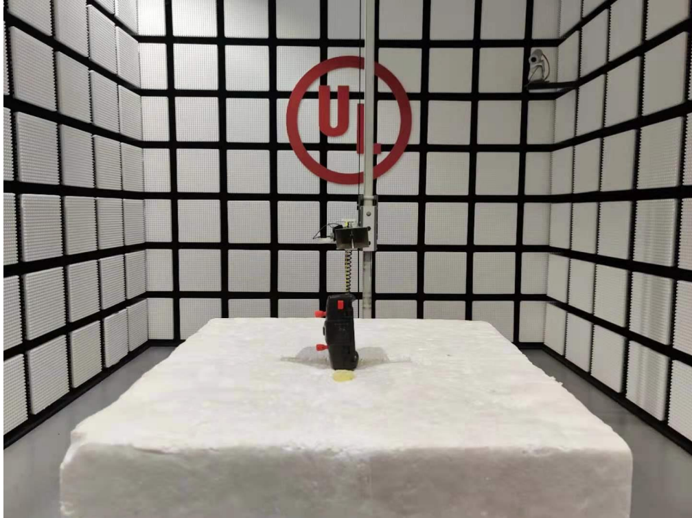
Radiated Disturbance Setup (Above 1 GHz – Z axis)
