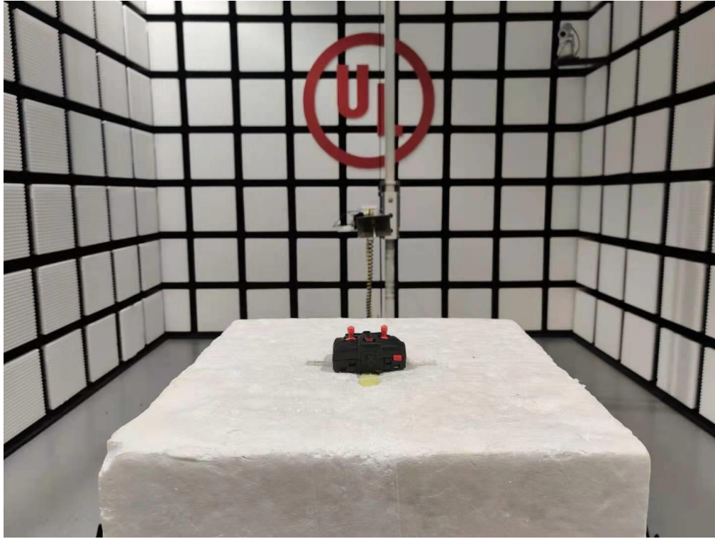
Radiated Disturbance Setup (Above 1 GHz – Y axis)
