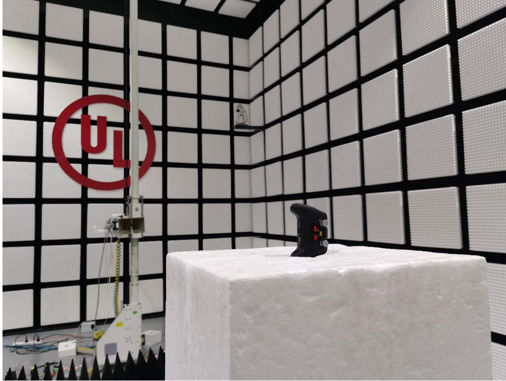
Radiated Disturbance Setup (Above 1 GHz – Z axis)
