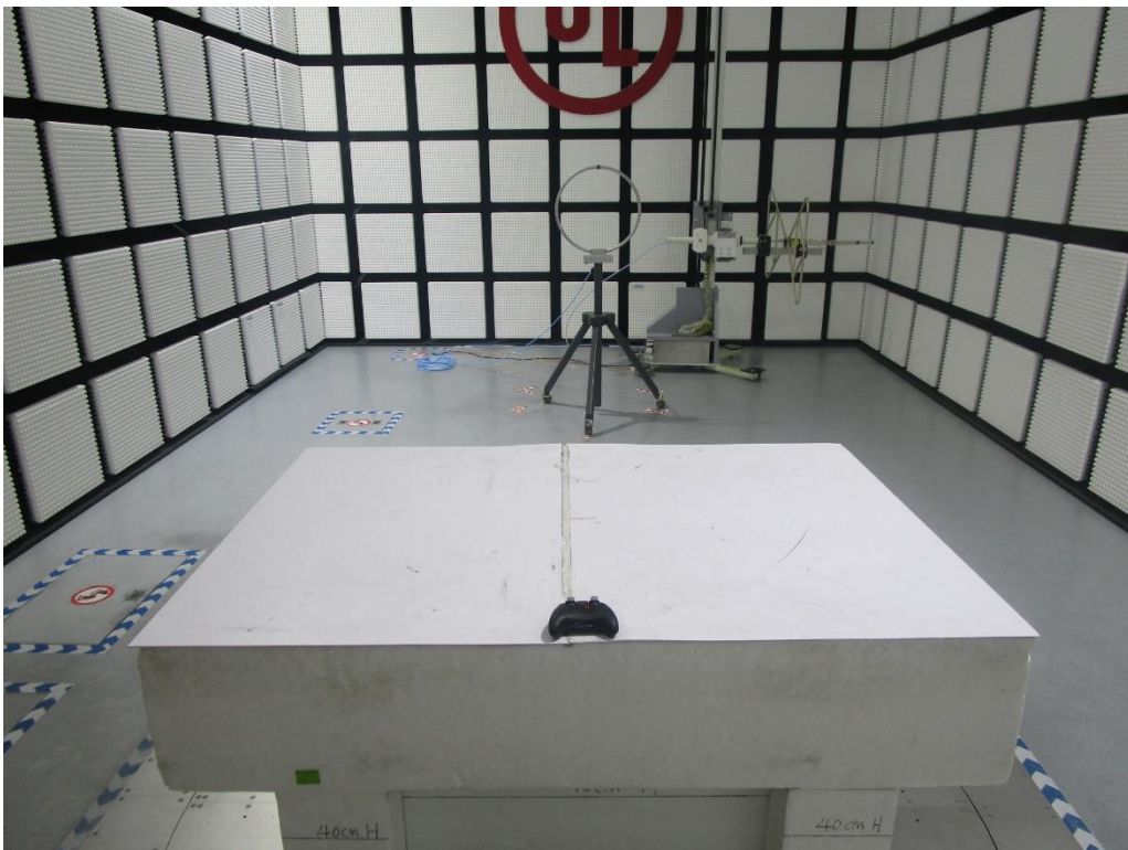
Radiated Disturbance below 30 MHz
