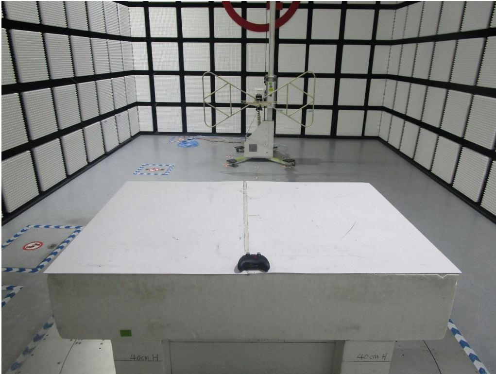
Radiated Disturbance below 30 MHz
