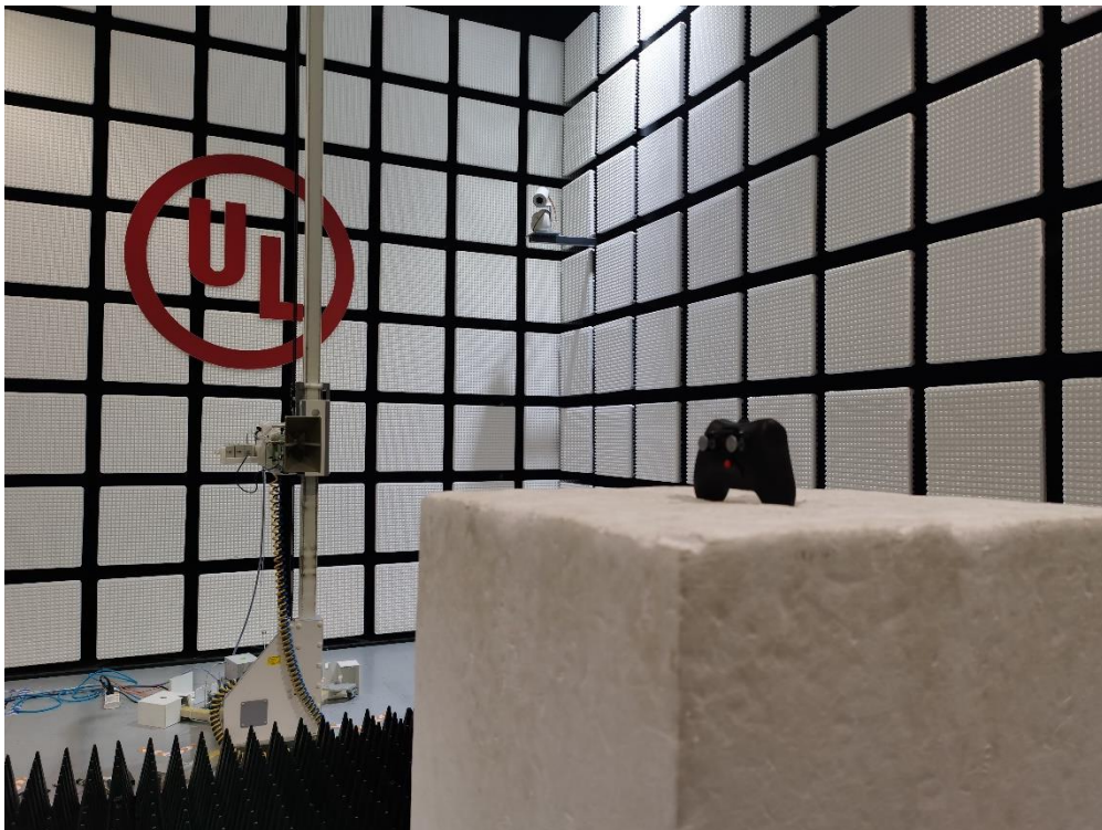
Radiated Disturbance Setup (Above 1 GHz – Y axis)
