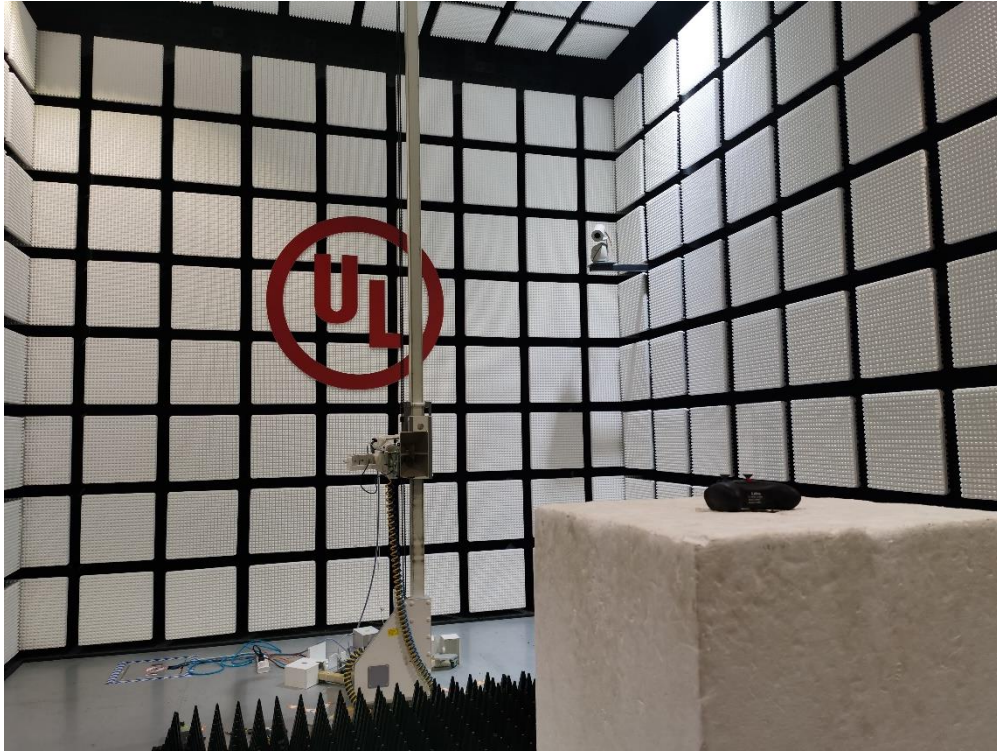
Radiated Disturbance Setup (Above 1 GHz – Y axis)
