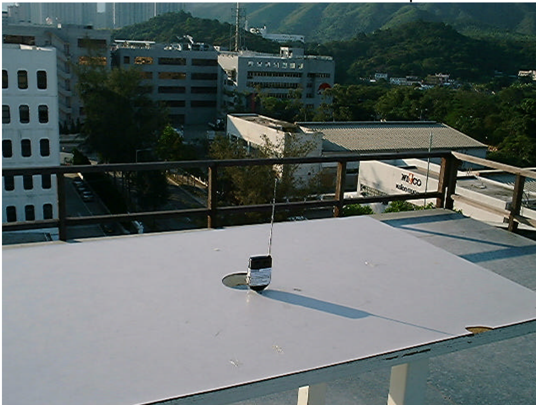
Measurement of Radiated Emission Test Set Up
