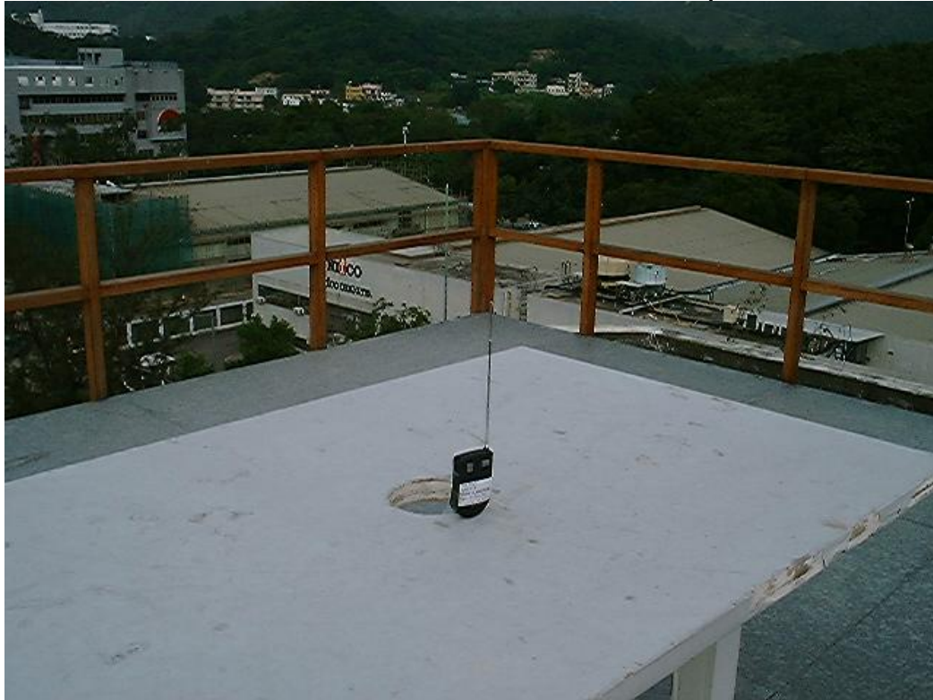
Measurement of Radiated Emission Test Set Up
