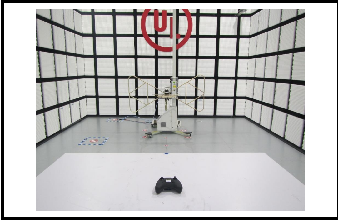
RADIATED RF MEASUREMENT SETUP (30MHz ~ 1 GHz)
