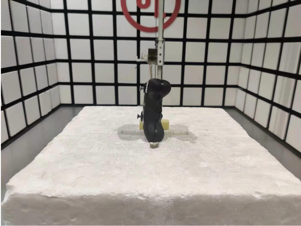
Radiated Disturbance Setup (Above 1 GHz – Z axis)
