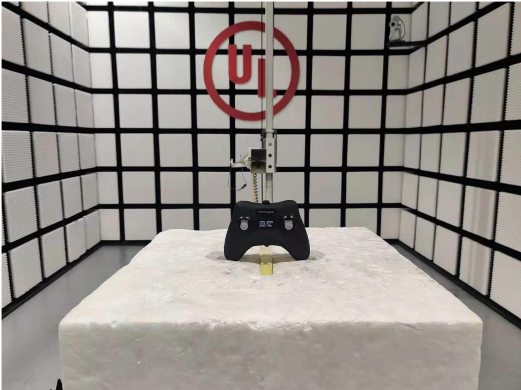
Radiated Disturbance Setup (Above 1 GHz – Y axis)
