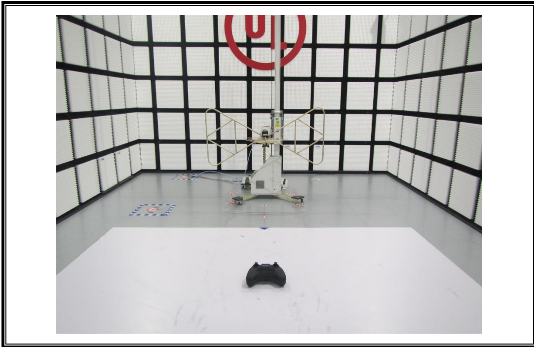
RADIATED RF MEASUREMENT SETUP (30MHz ~ 1 GHz)
