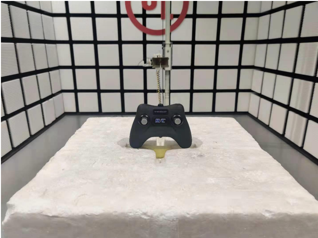
Radiated Disturbance Setup (Above 1 GHz – Y axis)
