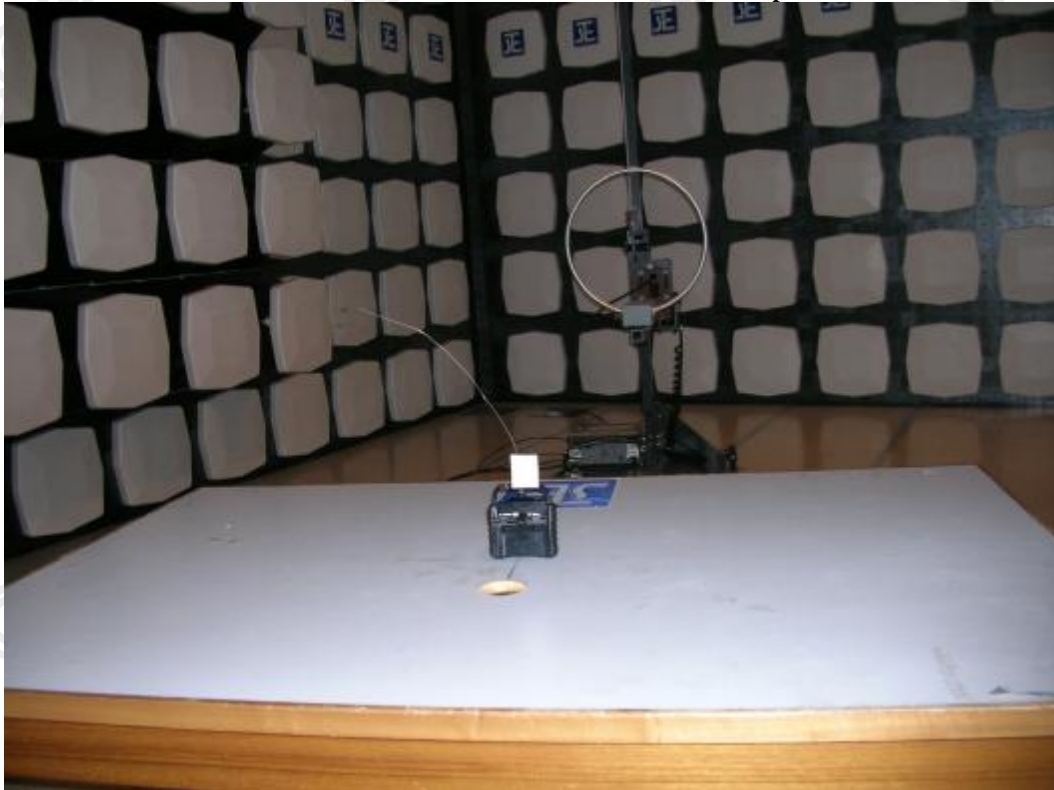
Measurement of Radiated Emission Test Set Up
