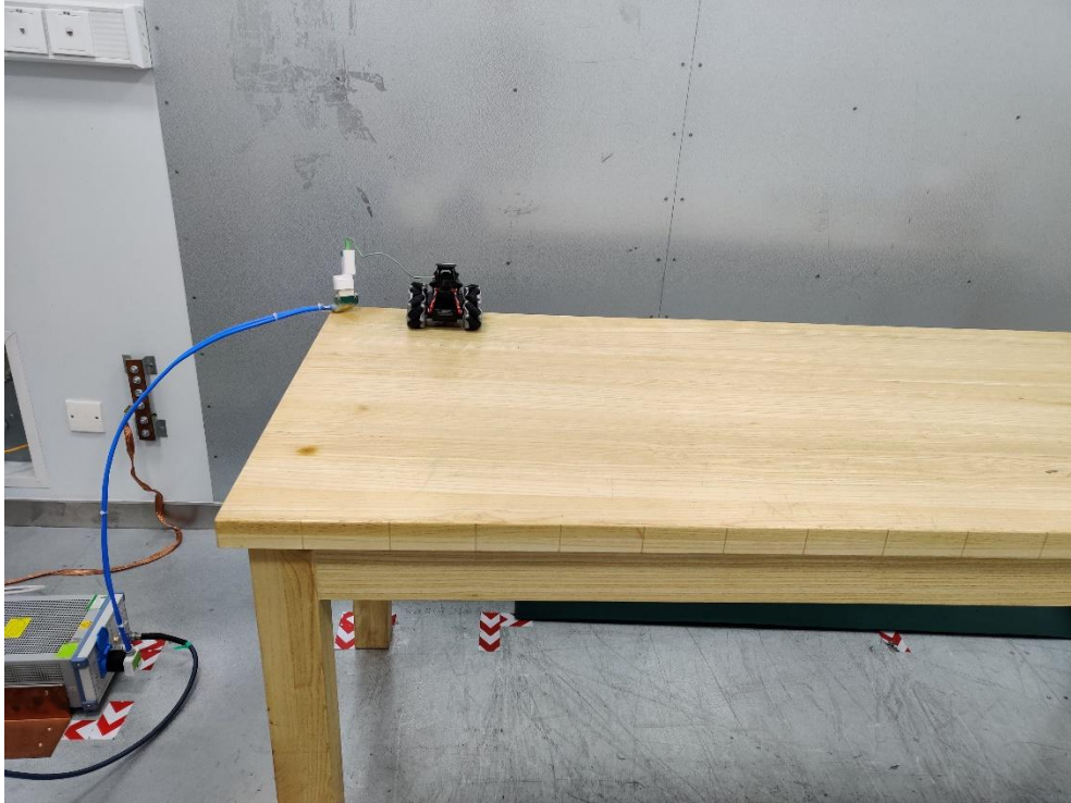
Radiated Emissions below 1GHz test setup photo Charging
