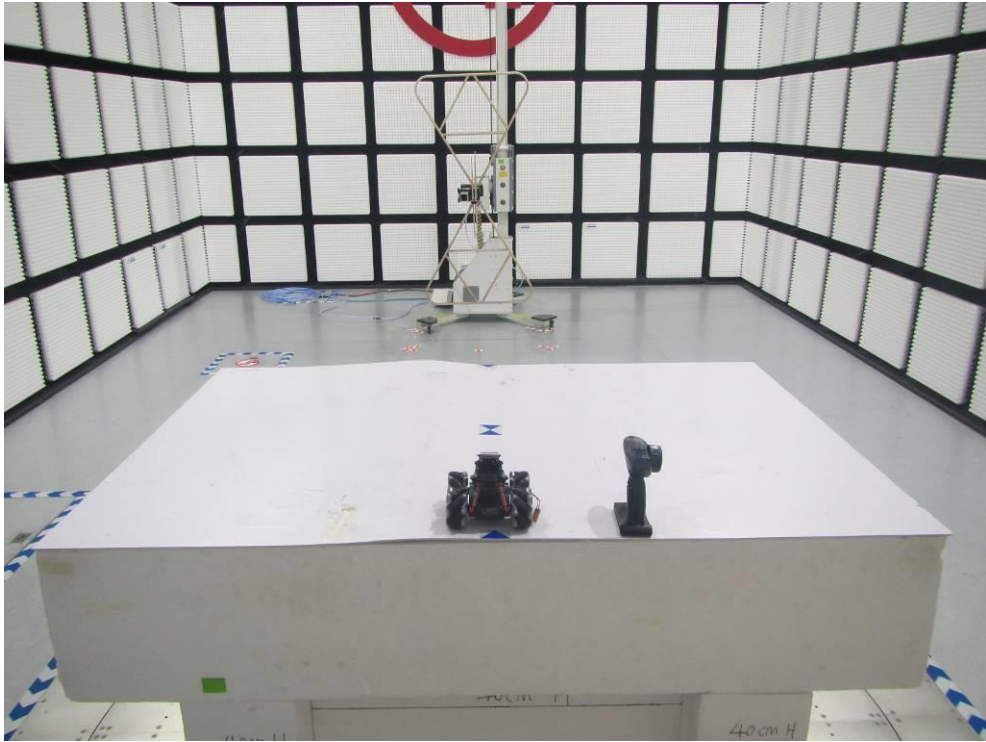
Radiated Emissions above 1GHz test setup photo
