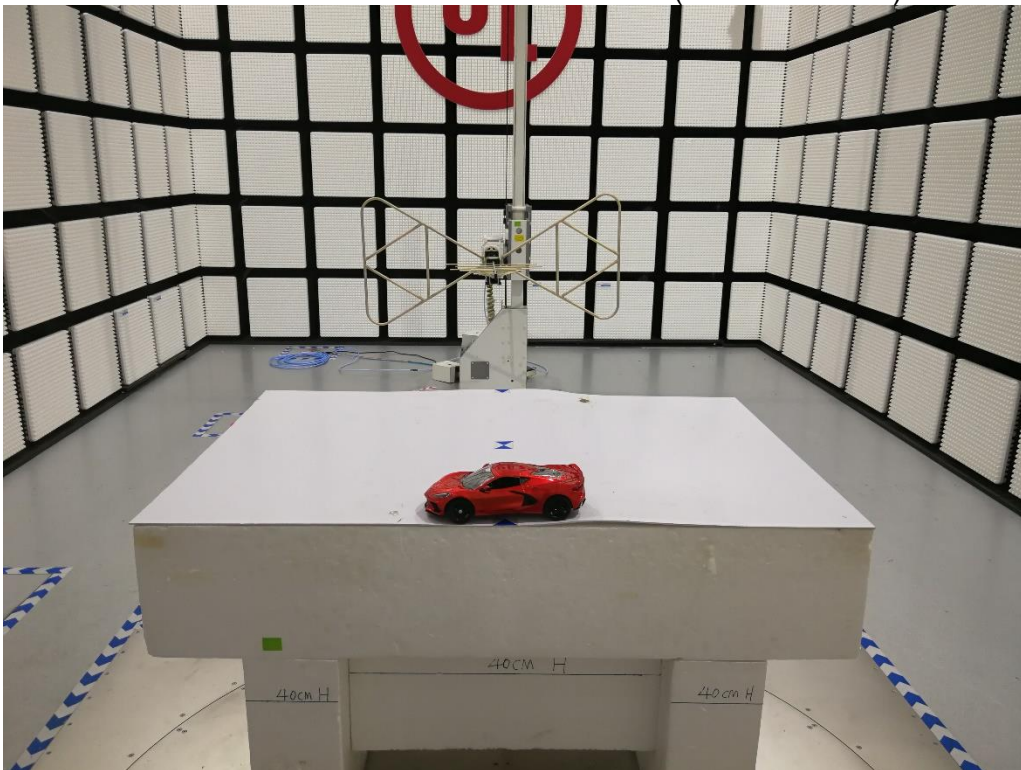
RADIATED RF MEASUREMENT SETUP (30MHz ~ 1 GHz)
