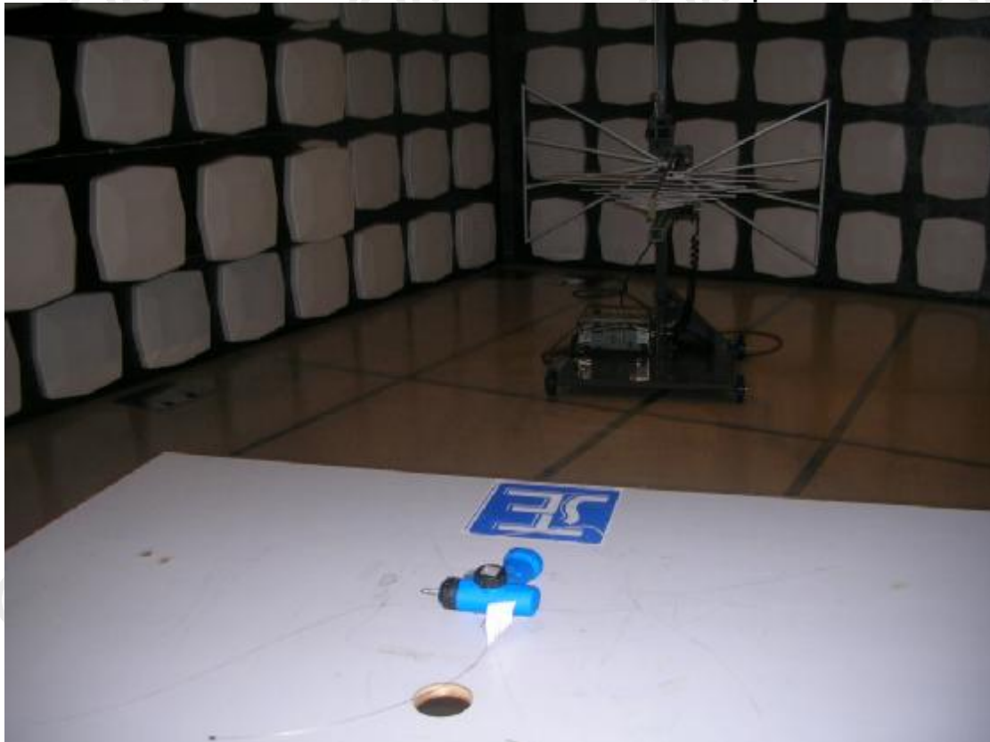
Measurement of Radiated Emission Test Set Up
