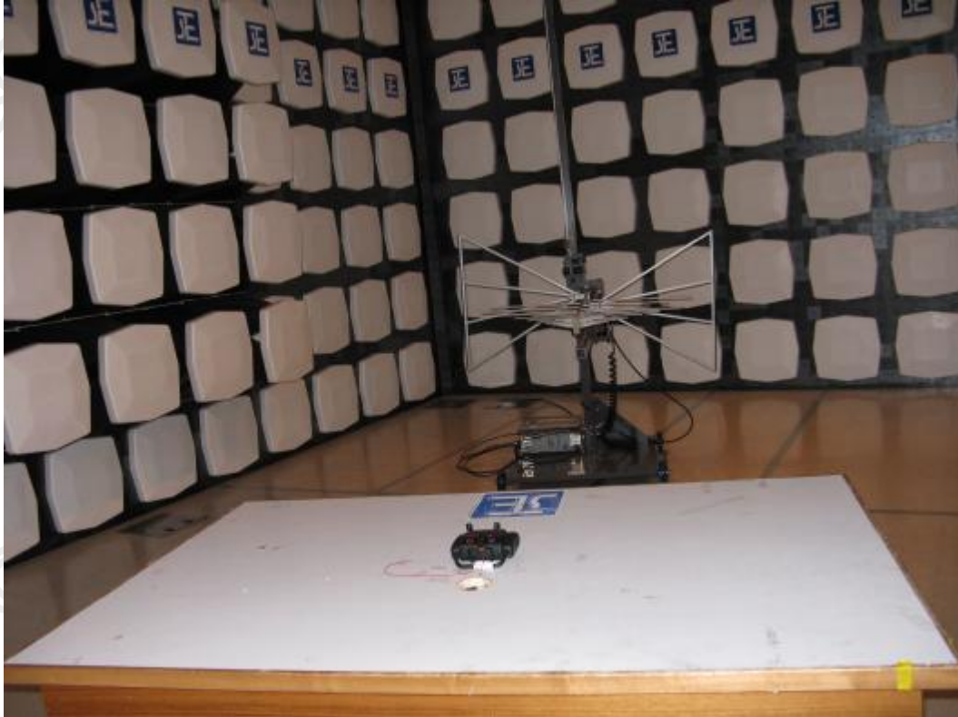
Measurement of Radiated Emission Test Set Up
