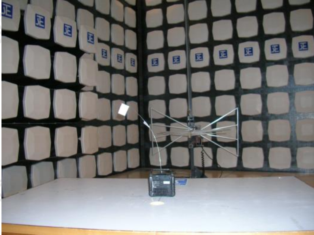
Measurement of Radiated Emission Test Set Up
