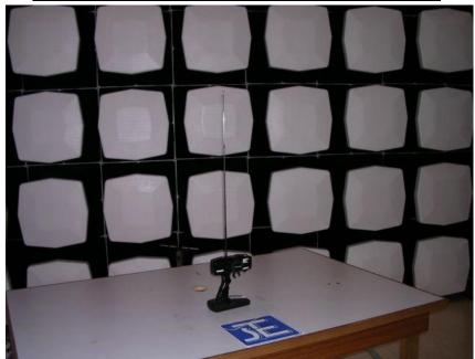
MEASUREMENT OF RADIATED EMISSION TEST SET UP
