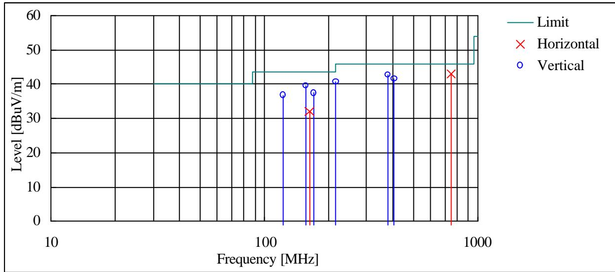
Notes: The test is performed in a distance of 3 m.
