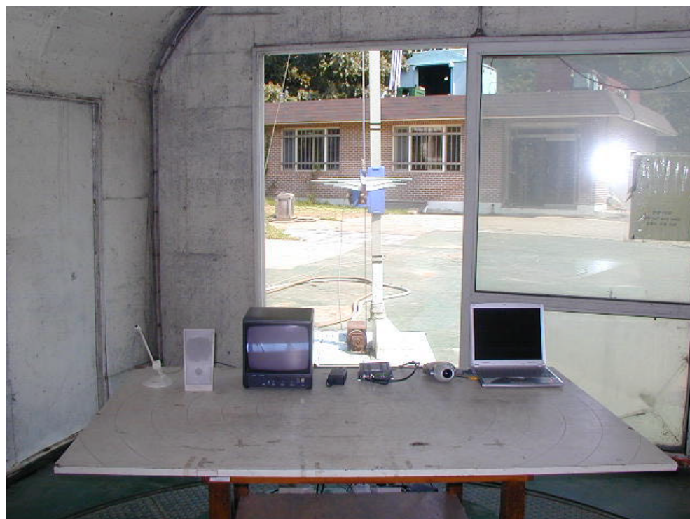
RADIATED EMISSION SETUP PHOTOGRAPH - FRONT VIEW ( 300- 1000 MHz )
