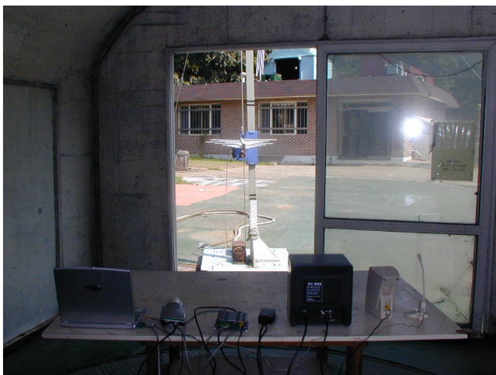
RADIATED EMISSION SETUP PHOTOGRAPH - REAR VIEW ( 300 - 1000 MHz )
