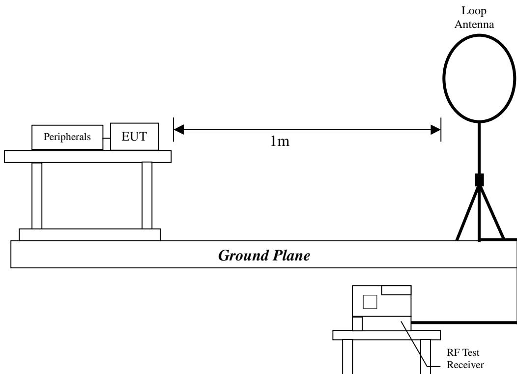
The signal is maximized through rotation and placement in the three orthogonal axes. The EUT and its peripherals are placed on a turn table which is 0.8 meter above ground. The turn table can rotate 360 degrees to determine the position of the maximum emission level. The EUT was positioned such that the distance from antenna to the EUT was 1 meter.
