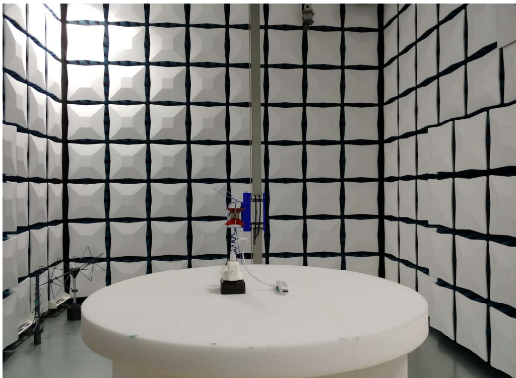
Set-up for Radiated Emission Above 1GHz
