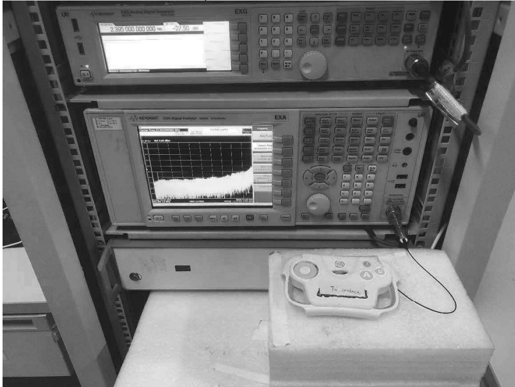
Set-up for Conducted RF test
