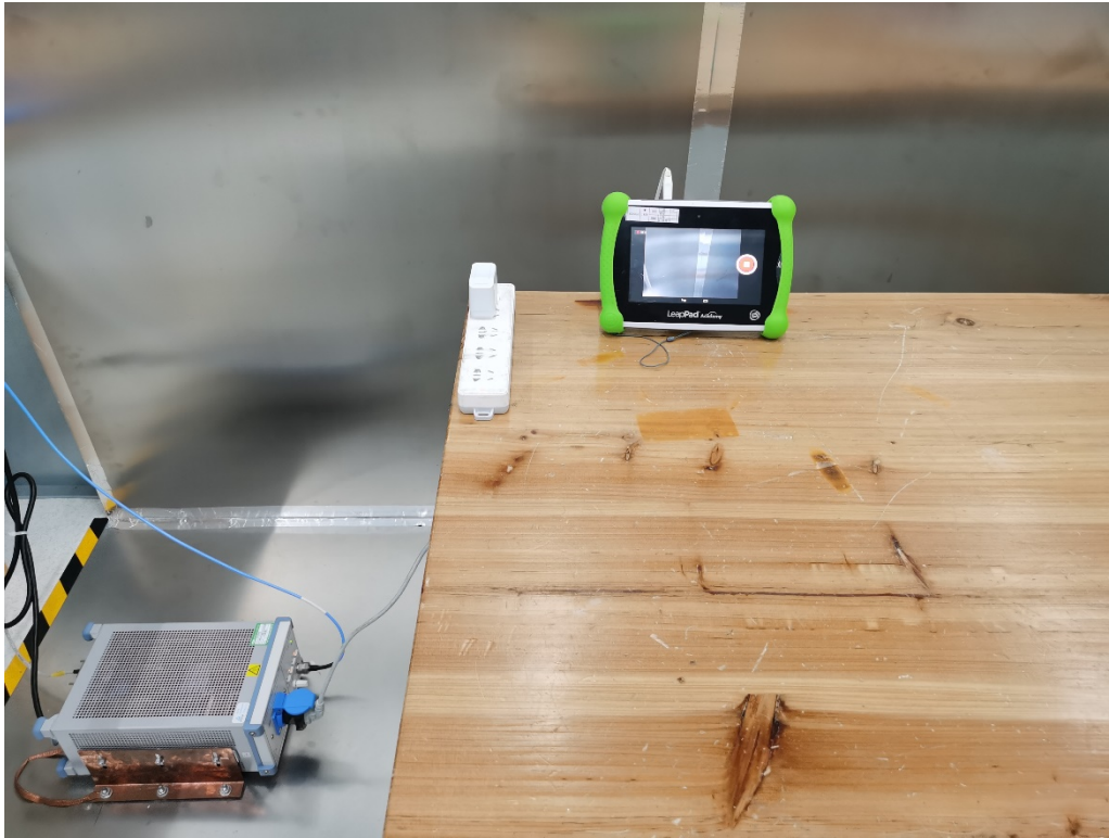
Photograph 5: Set-up photo for Conducted Emission on AC Mains
