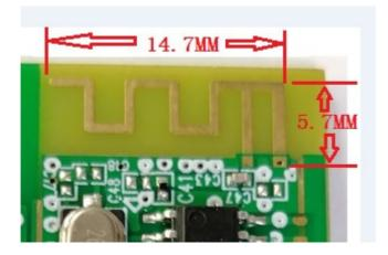
Figure 1 Physical dimension (mm)
