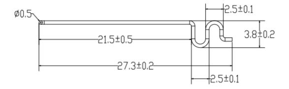
Figure 1 Physical dimension (mm)
