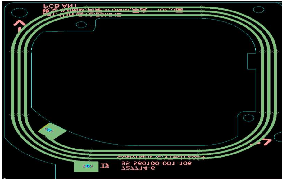
Figure 2.2 PCB antenna for RFID module
