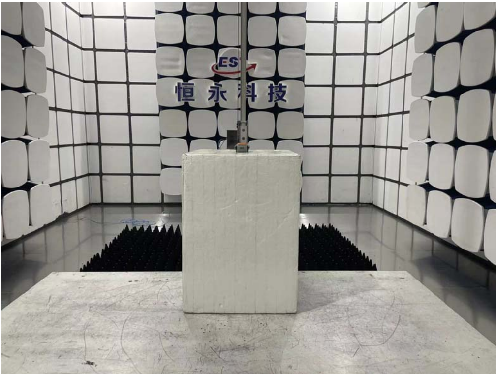
Radiated Test (Above 1GHz)
