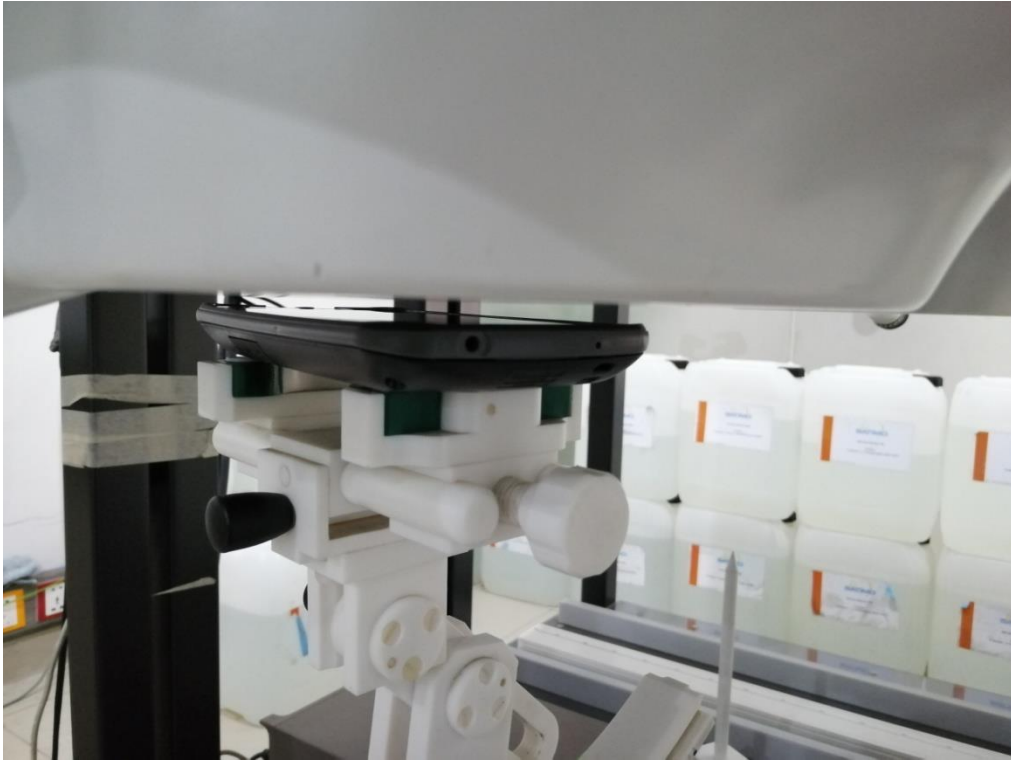
Body Front side(separation distance is 5mm)
