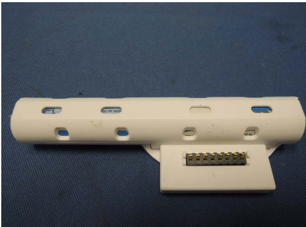
Figure 4 - 2.4V 2000mAh rechargeable battery package 1 back view
