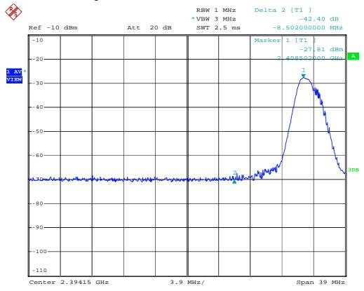
For 2400MHz bandedge checked with 2409MHz frequency operated, the delta shown at the plots are 27.7dB for peak detector mode and 42.4dB for Average detector mode.
