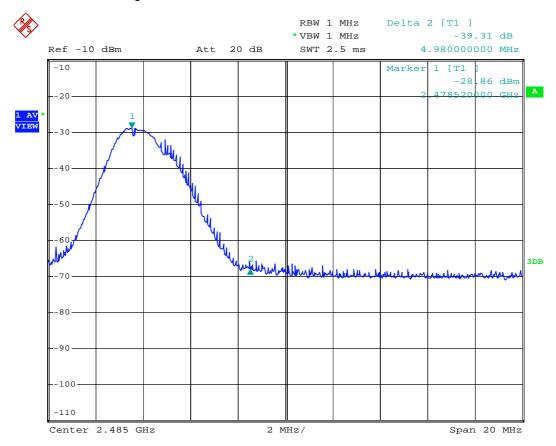
For 2483.5MHz bandedge checked with 2479MHz frequency operated, the delta shown at the plots are 26.5dB for peak detector mode and 39.3dB for Average detector mode.
