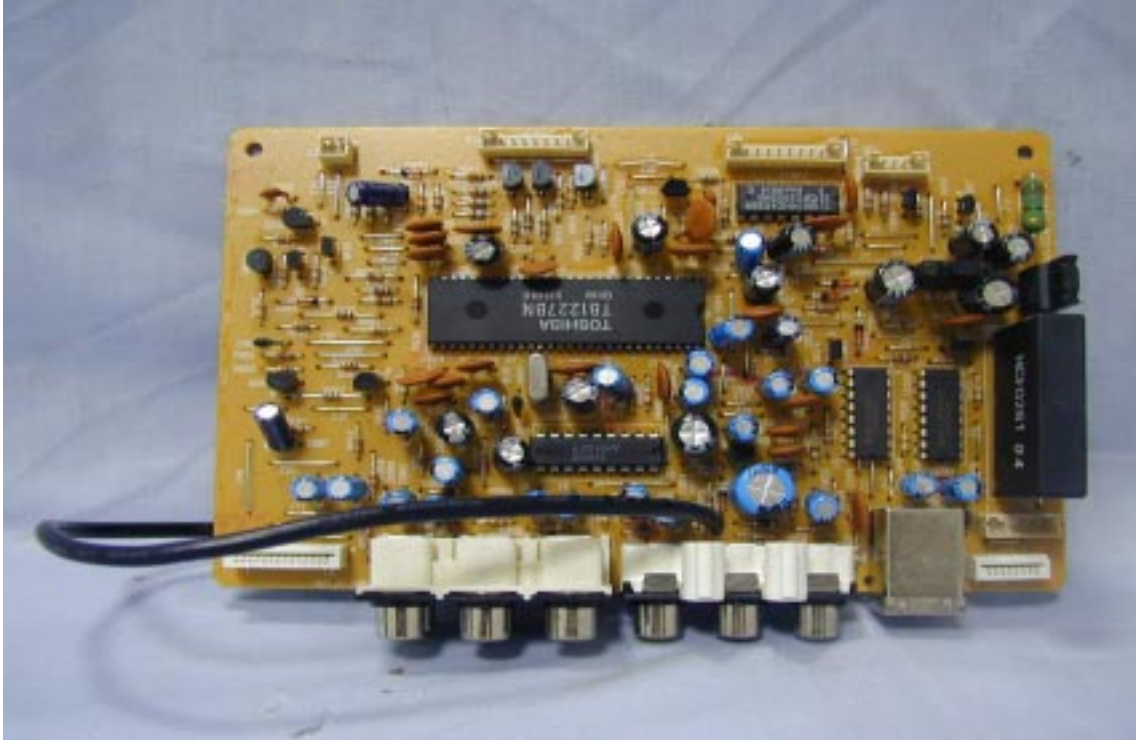
Component Side View of I/O Board
