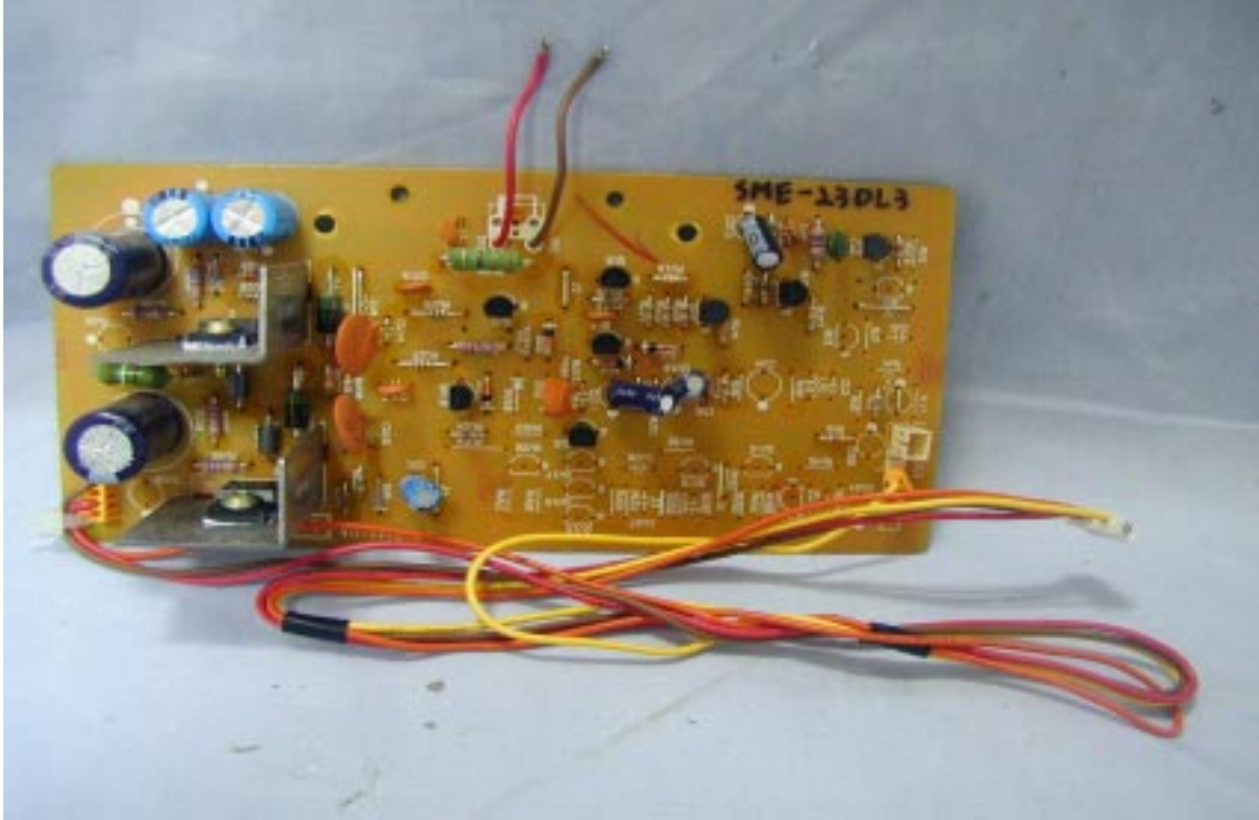
Component Side View of V & H Sync. Board
