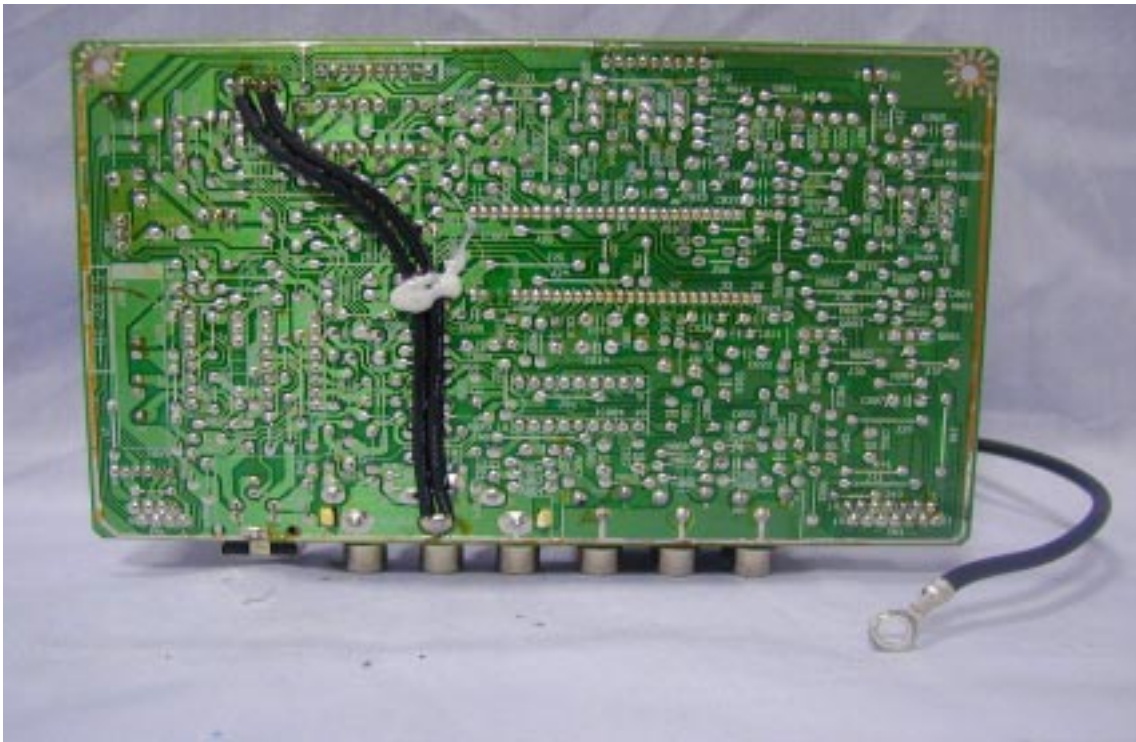
Solder Side View of I/O Board
