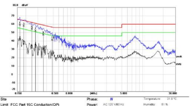
Limit: FCC Part 15C Conduction(QP)
