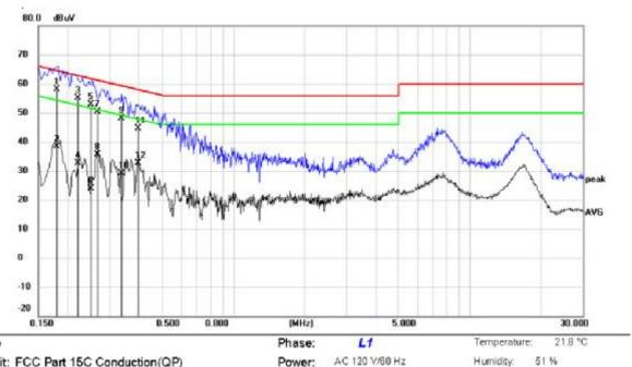
Limit: FCC Part 15C Conduction(QP)
