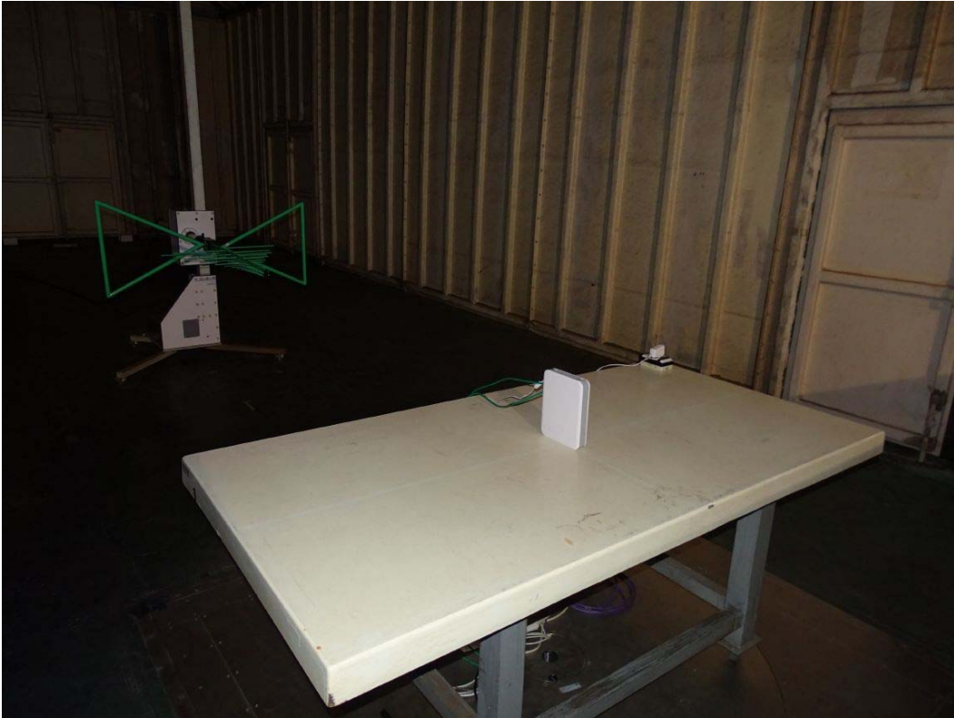
Front View of Radiated Test
