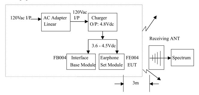
Three channels were tested: CH01, CH10 AND CH20 Measurements were taken by using both horizontal and vertical antenna polarization, and the antenna was raised and lowered from one to four meters to find the worst emission levels.
