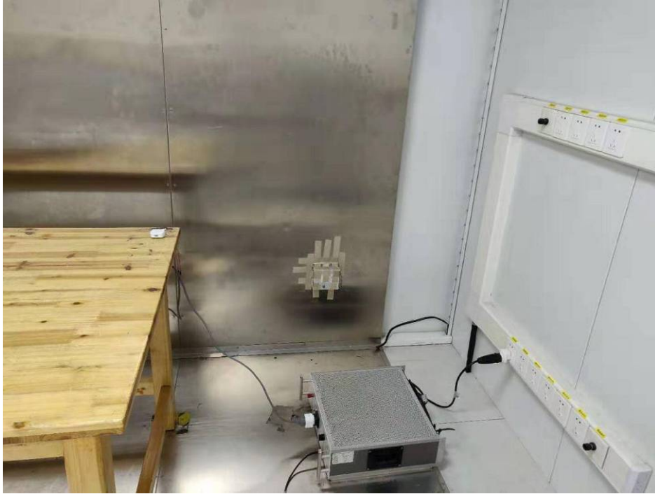
Radiated Spurious Emissions From 30MHz-1000MHz
