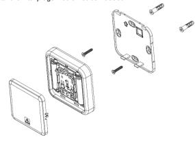
iv. Position the rear cover on the wall and turn the two screws into the wall (or wall plugs). DO NOT fasten too tightly as the rear cover might be damaged. Then replace the main body and the front cover.
