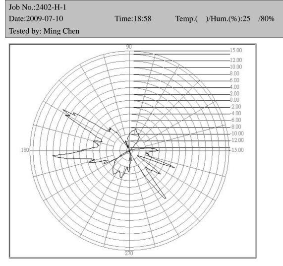
Center freq.(MHz): 2402 Max gain(dBi):-6.44 Polarization : H Plane Min gain(dBi):-38.55
