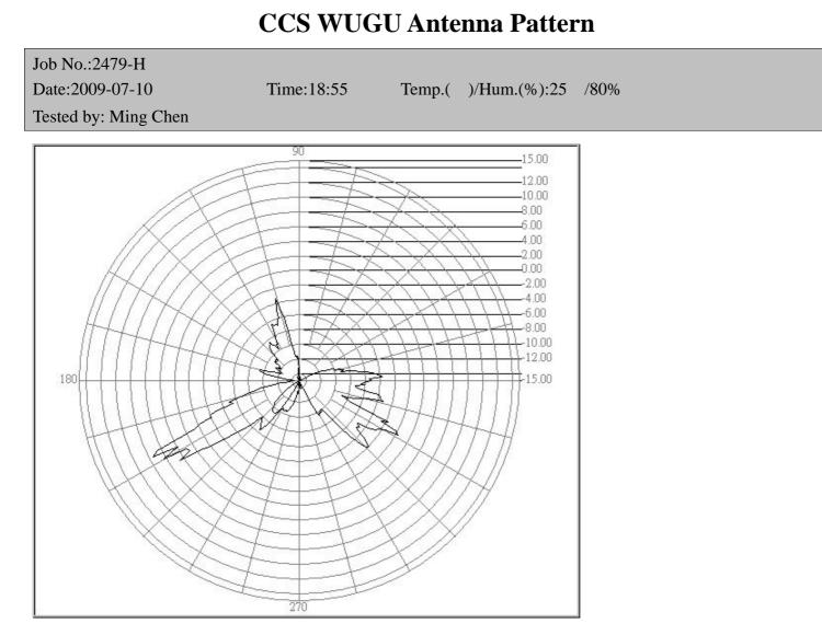
Center freq.(MHz): 2479 Max gain(dBi):-9.37 Polarization : H Plane Min gain(dBi):-37.42
