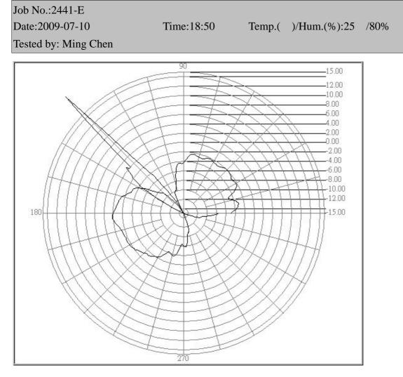
Center freq.(MHz): 2441 Max gain(dBi):0.24 Polarization : E Plane Min gain(dBi):-50.29
