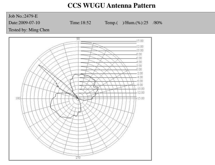
Center freq.(MHz): 2479 Max gain(dBi):0.19 Polarization : E Plane Min gain(dBi):-42.20
