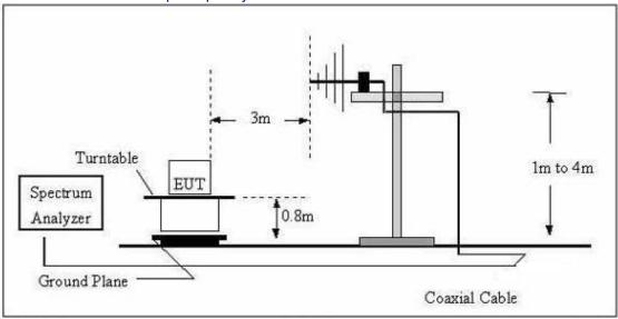
(C) Radiated Emission Test-Up Frequency Above 1GHz
