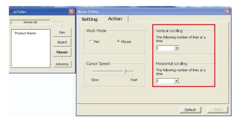
The mouse wheel supports vertical and horizontal scrolling, so you can set up the number of lines at a time while scrolling from 1 to 3 lines.
