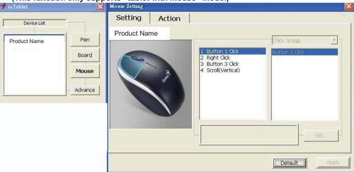
All the programmable mouse buttons are shown on the left side of the menu. Click on any of them to find out the location and the programmable setting. You may re-program any button from the drop down menu below the tablet picture.
