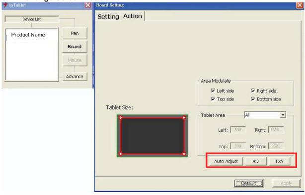
This tablet can be adjusted according to your LCD display.
