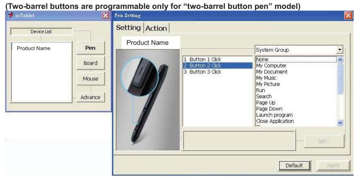
You may re-program the functions of the pen tip and the two-barrel buttons by selecting the button name from the drop down menu and assign a command of a traditional three-button mouse to it. The programmable group includes:
