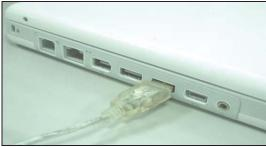
Connect the tablet USB interface to your MAC after you have finished the driver installation and restarted the system: Install the driver first before plugging the tablet into your MAC.
