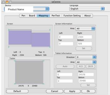
**B.** Define the tablet's working area and mapping range on your LCD screen. It also supports screen size switching (4:3/16:9) function.
