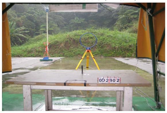
Horizontal Polarization and the EUT (30MHz~1GHz)
