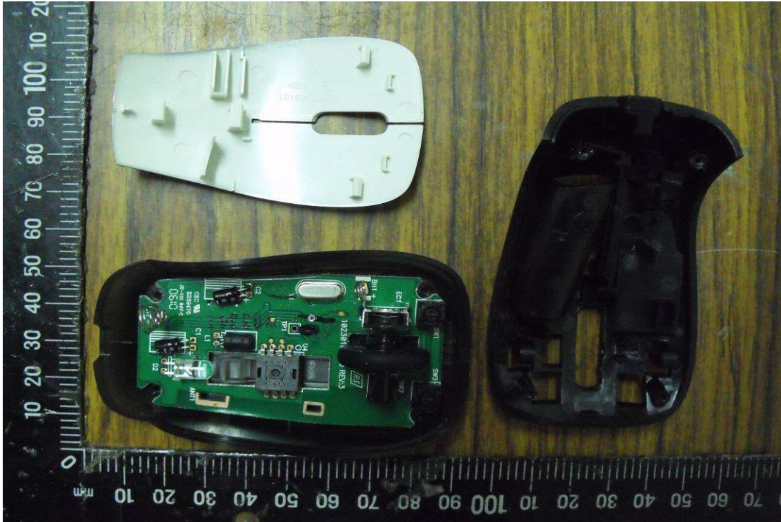
Inside View of New EUT
