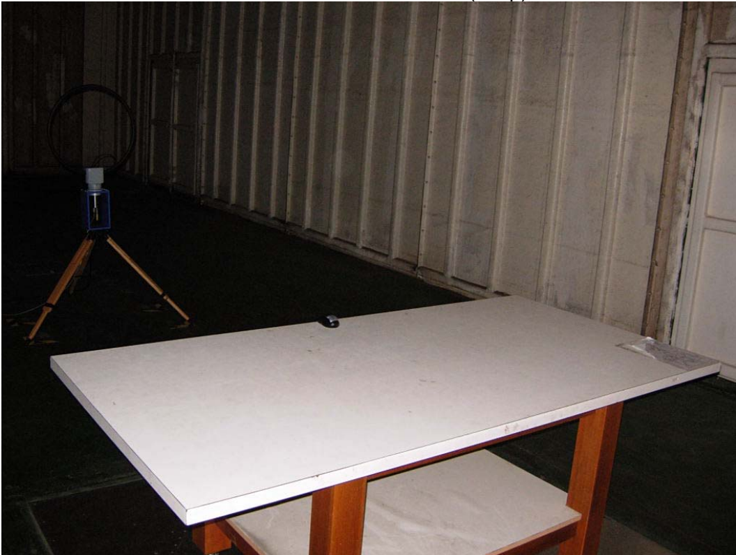
Front View of Radiated Test (Loop)
