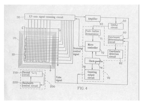
End of these states micro-controller (72) will rescan the X-Y axis antenna Area and wait the PEN ( or mouse PUCK ) feedback signal for next cycle .
