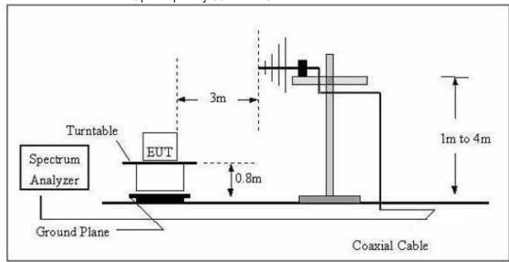
(C) Radiated Emission Test-Up Frequency Above 1GHz
