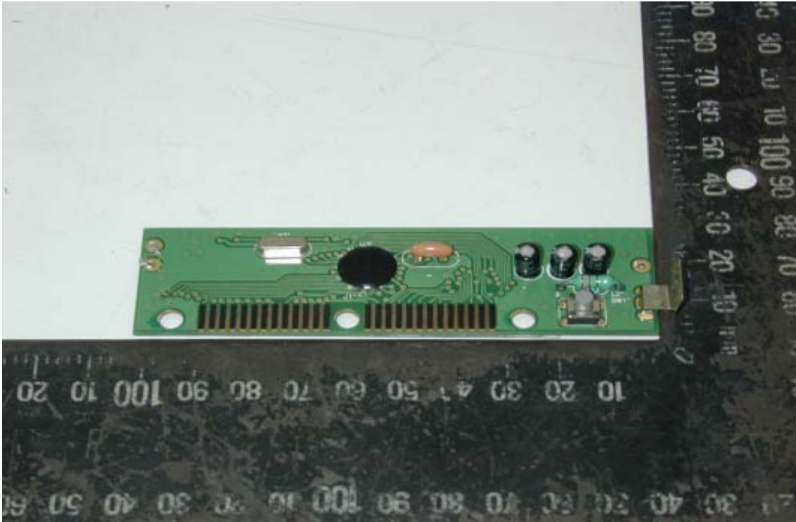
Solder Side of Main Board
