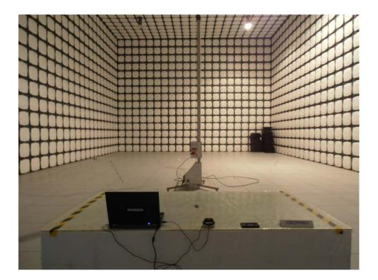
2 Set-up for conducted emission test
